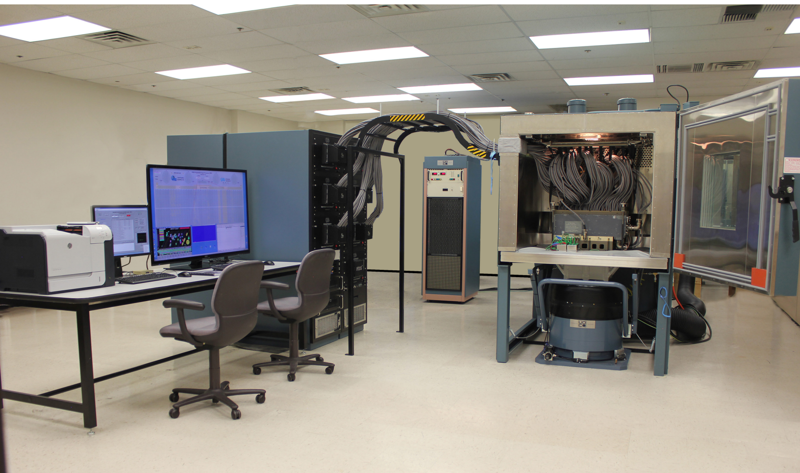
Total Quality Systems' Intermittent Fault Detection and Isolation System (IFDIS)
